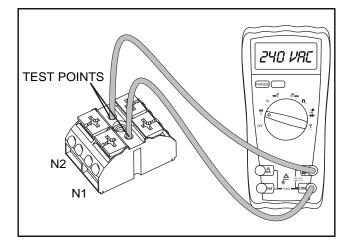
Figure 9. Terminal Block Test Points
